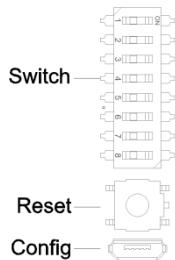
Switch: The DIP switch is used to set the name of Profinet device.
