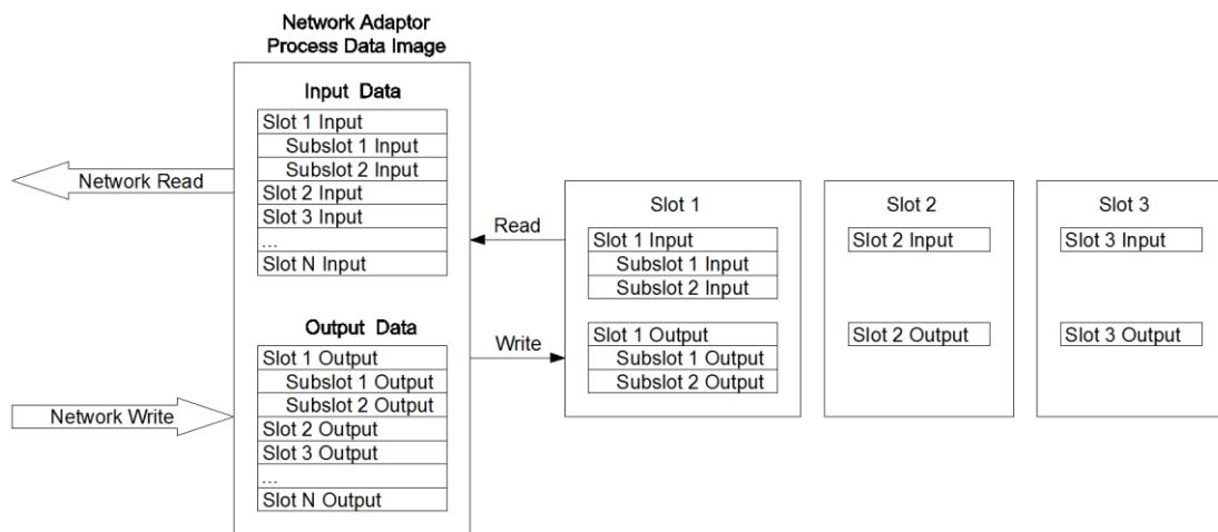
The maximum number of input bytes of the Profinet network adapter is 1440 bytes, and the maximum number of output bytes is 1440 bytes.
