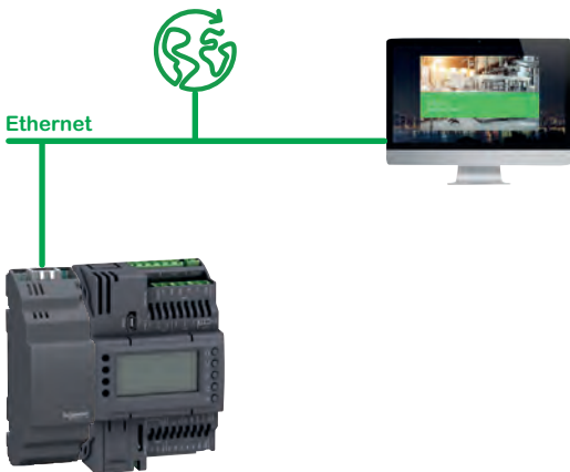
M172 Optimized logic controller linked to Ethernet via the TM171AETH or TM171AETHRS485 communication module
