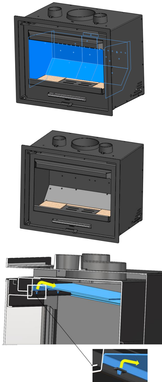
Figure No.9 - Dismantling the ADOUR steel deflector
