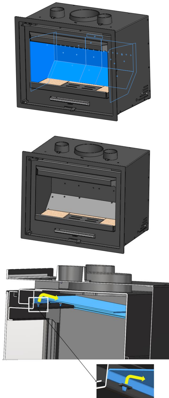
Figure No.9 - Dismantling the ADOUR steel deflector
