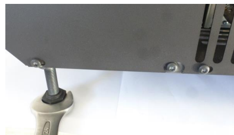
Figure No.4 - Close up of the 24 mm wrench for adjusting the legs
