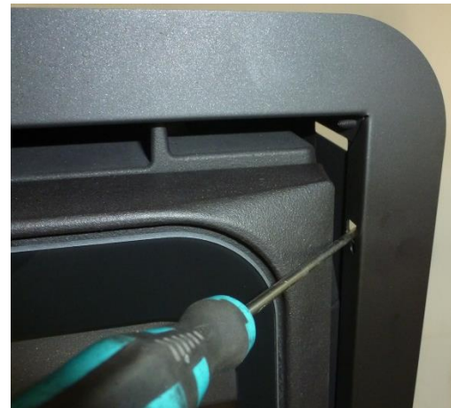
Figure No.12 - How to bend the tabs
