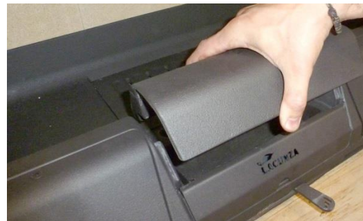
Figure No.2 - Removing the separator
