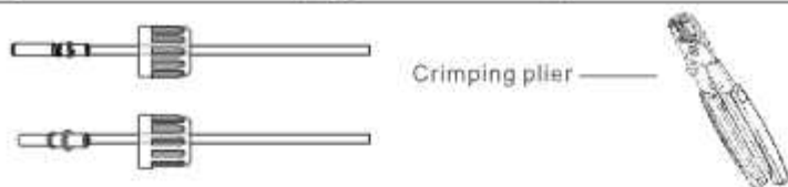
Pic 3.4 Crimp the contact pin to the wire
