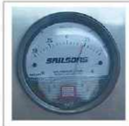
Pressure Meter Display the pressure of work zone.
