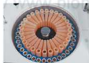
Reagent Tray Refrigerated tray with independent switch.
