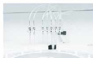
Washing Probe Independent 7-step washing system.
