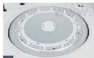
Reaction Tray 37±0.2°C, real-time monitor.
