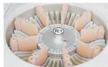
Reagent Tray 2~8°C cooling for 24 hours.
