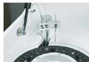
Washing Probe Independent 3 -step washing system.
