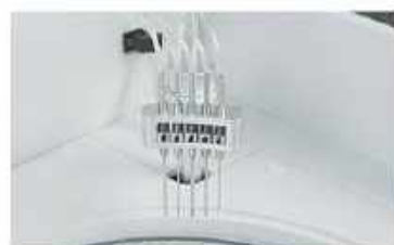
Washing Probe Independent 5-step washing system.
