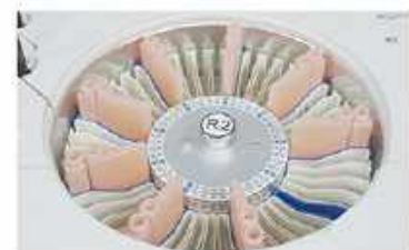
Reagent Tray 2~8°C cooling for 24 hours.
