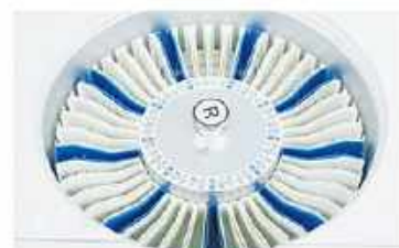
Reagent Tray 2~8°C cooling for 24 hours.
