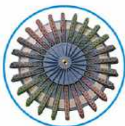
Rotor: Capacity: 24cards Speed: 4000 rpm RCF: 1459 xg
