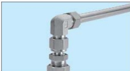
4. Connect union elbow to male adapter by tightening the Hy-Lok nut while keeping the elbow in the desired direction. Then install the tubing into the other end of elbow.
