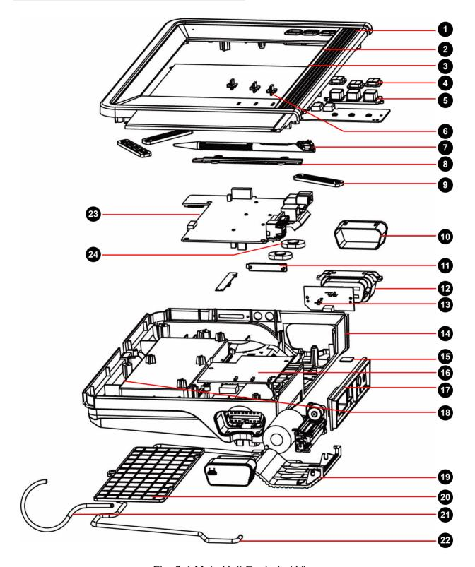
Fig. 3-1 Main Unit Exploded View
