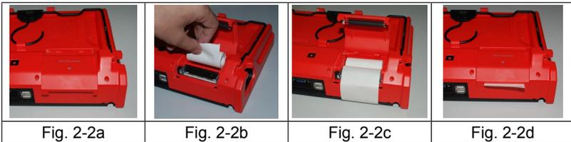
Fig. 2-2 Installing paper
