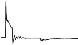
Secondary circuit resistance is too large
