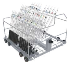
Full frame injection module FA-Z11 ▪38 pipettes can be loaded in three layers ▪1st Row:10pcs 10-100ml pipettes,H550mm ▪2nd Row:14pcs 10-25ml pipettes,H500mm ▪3rd Row:14pcs 1-10ml pipettes,H440mm ▪H373, W531, D582mm
