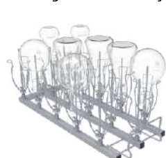
Injection Module 10 injections FA-K11/1 ▪For 250-500ml Erlenmeyer flasks, Reagent bottle,Blue cap bottle,Volumetric flask and so on. ▪Injector nozzle: \phi 6 \times H130 mm ▪H179, W240, D505mm Holder's height can not adjustable
