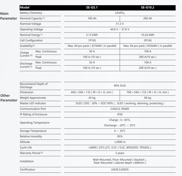
[1] Test conditions :  $25^{\circ}C \pm 2^{\circ}C$ , at beginning of life, 0.2C charge & 0.2C discharge,100% DOD.
