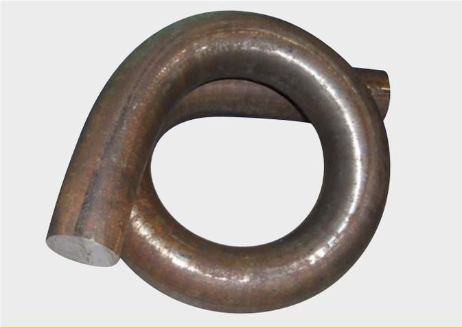
Rundmaterial ● Ø 50 mm (Sondermaschine)
