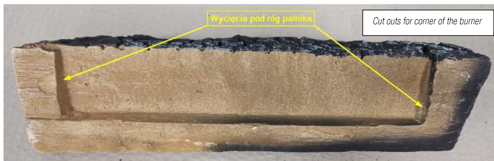
Picture 31. Incisions in items 2 and 3 facilitate laying in corners of the burner.
