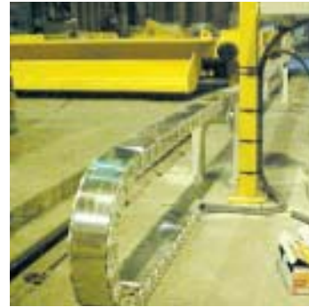
Provides a safe process: Boa steel chain with covers in a steel mill.
