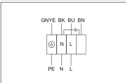
**Wiring diagram No. 3 (1~230V)**
