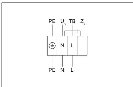
**Wiring diagram No. 4 (1~230V)**
