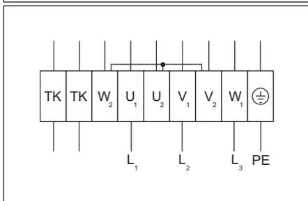
**Wiring diagram No. 2 (Y - 3~400V)**
