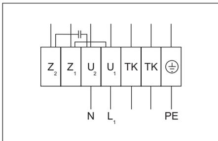
**Wiring diagram No. 1 (1~230V)**
