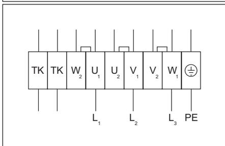
**Wiring diagram No. 2 (Δ - 3~230V)**
